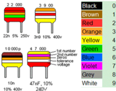
Fig 6: Color coded capacitors and labeled capacitors
